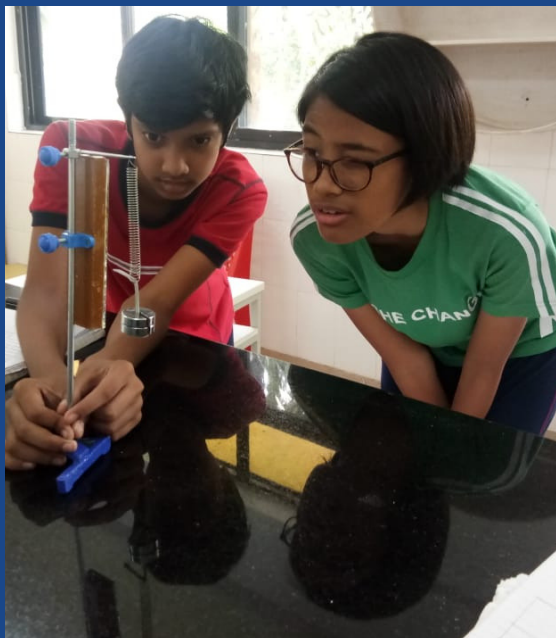
Year 10 Physics students performing experiment on Hooke's law to find the constant of a spring.
